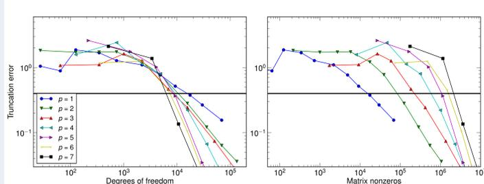
Figure: Two measures of cost for 3D high-order finite element methods. The dark line represents an example suitable accuracy. Finite element methods of order  $p$  involve element matrices of size  $p^3 \times p^3$ . Since solver cost is almost always superlinear in the number of nonzeros in the Jacobian, high-order methods that involve assembling the true Jacobian are rarely economical.
